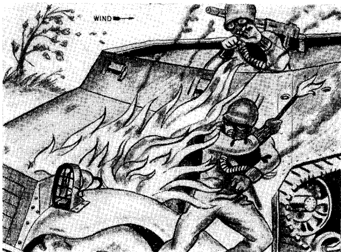
FIGURE 24.—Do not burn from down wind side or you may be seriously burned by flames and by the heavy vapor concentration driven off.
